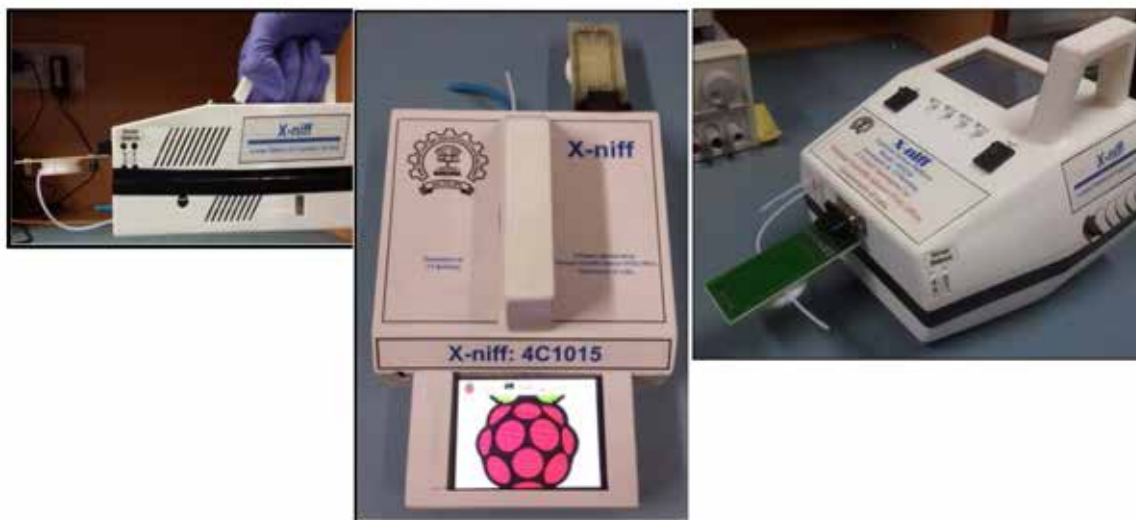
Fig. 4 The handheld vapour-phase explosive detection prototype, X-niff, developed by our group at IIT Bombay with support from the Principal Scientific Advisor's office, Gol.
